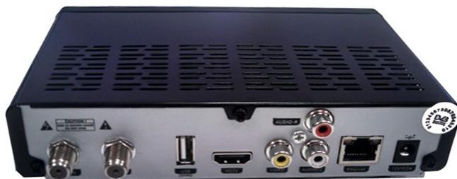
**EiTV CC Box** decoder has the ability to decode the ISDB-Tb signal and generate the composite format (NTSC / PAL-M) with the caption on line 21 and apply the LetterBox / PanScan video formats.
