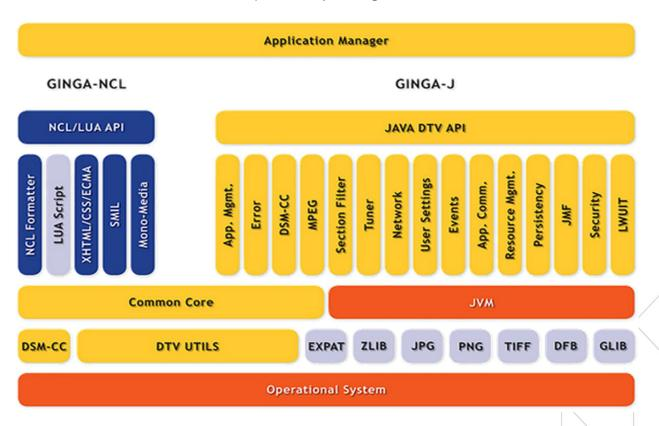
The Applications Manager controls the life cycle of high-level applications and communicates with the DSM-CC (data / object carousel), with the NCL formatter and the JVM (Java Virtual Machine).
